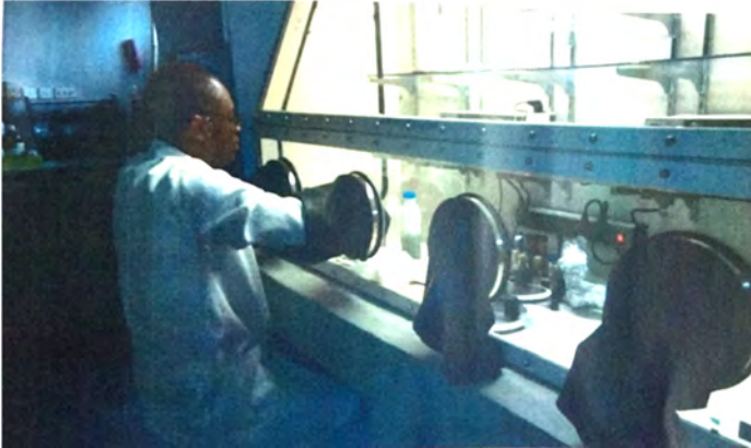
Plate. 3: A double chamber Anaerobic Box in use at the Central Instruments Laboratory (CIL), Uniport.
